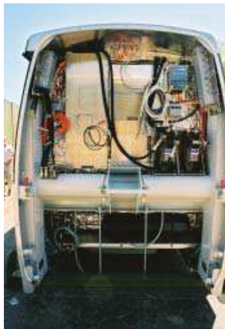
After taking delivery of the Swiss-made train cabins, Schwager Davis, Inc., performed wiring and final assembly of the vehicles on-site.
